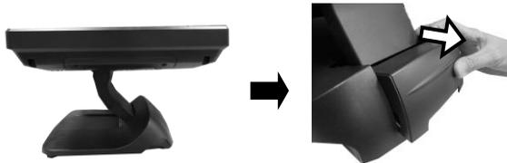
4.2 Support the screen with one hand holding onto its bottom edge. While pulling the lever backwards, move the display downwards until the lever is lifted off the hook as shown in the figure
