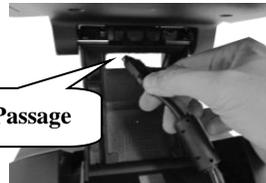
5. After tilting the screen all the way up, remove the bottom I/O cover to locate the bottom I/O plate.
