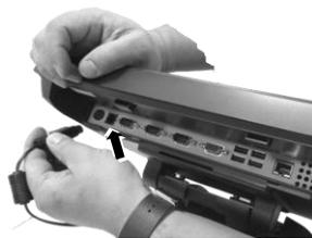
7. Tuck the extra cables inside the bottom I/O compartment, and then push back the cover to close it.
