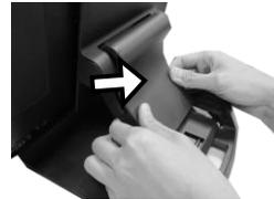
4. Tilt the terminal to the horizontal position. Then, thread cables through the cable passage.
