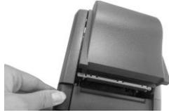
5. Remove the jammed paper, reinstall the paper roll, and then push back the cover to close the paper jams rescue compartment.
