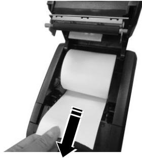
5. Make sure the loose end sticks out of the opening of the paper roll compartment. Then, close the top cover by gently pushing it back at the center of the top side of the cover with a click sound.
