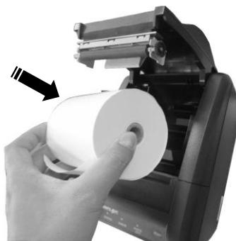
4. Unroll the thermal paper and drag the loose end of the paper till it extends towards the paper cutter.
